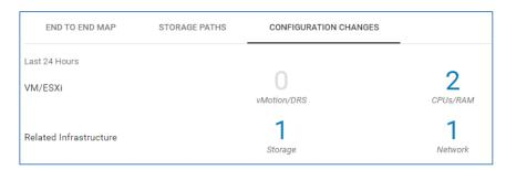
Selecting the number in the Configuration Changes view opens a window that displays details about the configuration change or changes. This allows the user to correlate configuration changes in the environment with potential performance impacts.
