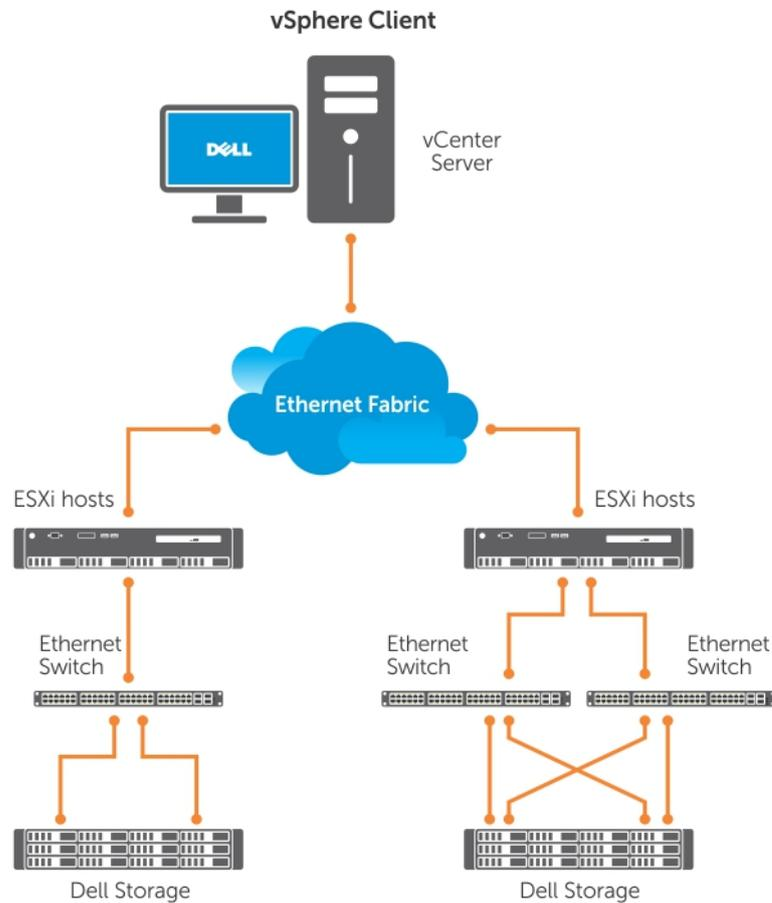
Figure 5. Configuring vSphere with iSCSI SAN
